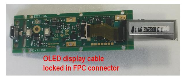
Now the cable is clamped and contacted.
