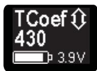
The selection of the correct wire-temperature-coefficient is very important for the correct operation of the mod, when temperature controlled vaping is selected.
