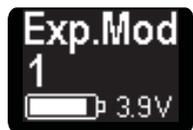
The dicoses no 6 can be used in 5 different modes. But in order to keep the menu as short and simple as possible, 3 of the 5 modes are only available, if the Expert-Mode is set to 1. The name is Expert-Mode, because the use of the additional operation modes requires additional knowledge about their functionality.
