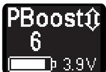
We recommend to set the normal power (not the boost) to much lower values, when using the periodic boost, because the average power is increased by the boosts and temperature gets higher therefore.
