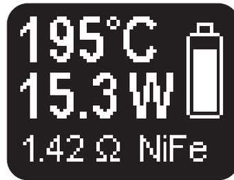
Battery status (including voltage drop during vape). Starts blinking at low bat and power reduction (see text)
