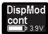
The display mode switches on and off the dynamic display of several parameters during and after the puff. The setting “cont” (continuous) will display values during and seconds after the vape. With “post” the values are displayed only after the puff and off disables the display.
