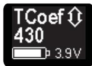
The selection of the correct wire-temperature-coefficient is very important for the correct operation of the mod, when temperature controlled vaping is selected.
