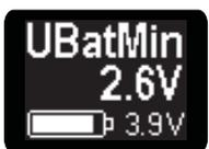
All dicodes devices have a functionality to adjust the minimum discharge level of the battery between 2.5V and 3.0V (older models 3.5V). Almost all available batteries on the market specify the minimum discharge level of 2.5V to 2.7V. If the user is unsure, whether her/his specific battery meets this specification, the level should be set to 2.7V.
