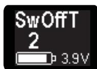
The time to automatic power off of the mod can be selected between 1 minute up to 60 minutes. We recommend to choose 2 or 5 minutes, because the mod is always immediately on and ready to vape, when the fire button is pressed. This provides the best utilization of the battery.
