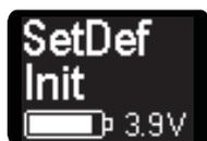
With “Set Defaults” it is possible to reset all settings to the delivery status. The reset is initiated by selecting the menu an pressing a button. To avoid unintended resetting the user has to confirm the procedure by again pressing the button when “confirm” is displayed. “Process” shows that the rest is performed.
